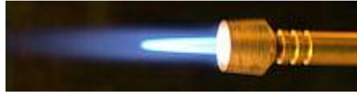
Fig2. Oxygen rich butane torch flame.
